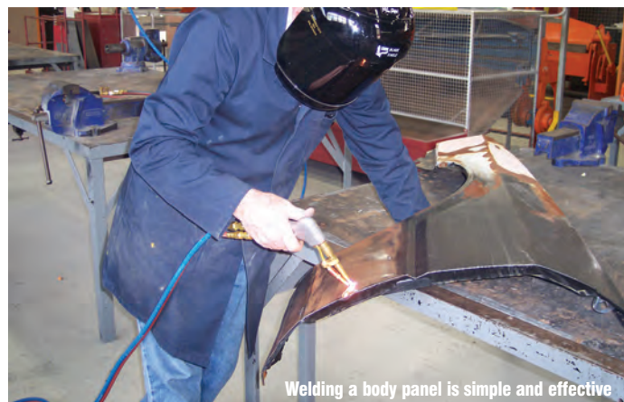
The DCH gives a neutral flame and a clean weld.
